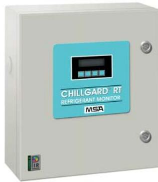
**The Chillgard® RT Photoacoustic Infrared Refrigerant Monitor** is the industry standard for refrigerant leak detection monitors, providing economical, low-level monitoring of refrigerant gases used in most refrigeration systems or chillers. The Chillgard RT Monitor utilizes very stable and highly-selective photoacoustic infrared (PIR) technology to sense refrigerant gases. The Chillgard RT Refrigerant Monitor
